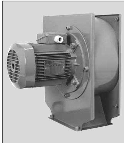
It is advisable to check that the machine outlets are not blocked, as this would cause the cooling air to be recycled, raising its temperature and possibly causing an abnormal rise in machine temperature.
